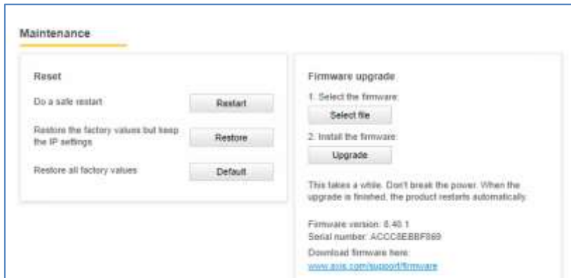
Axis camera setup: System Tab > Maintenance > Restart
